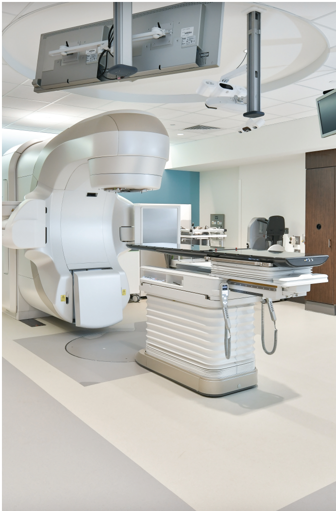
The linear particle accelerator treats cancer with precisely targeted high-energy beams of subatomic particles.
